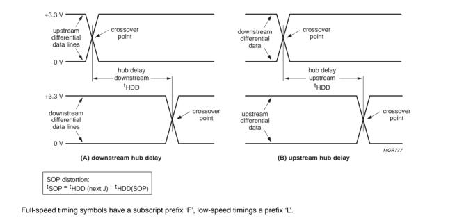
Fig 19. Hub differential data delay and SOP distortion.
